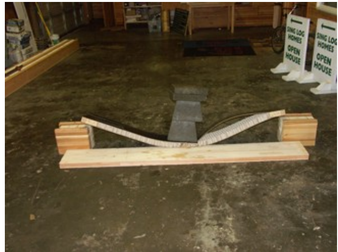
2" thick Paper Honeycomb panel collapsed under less weight
