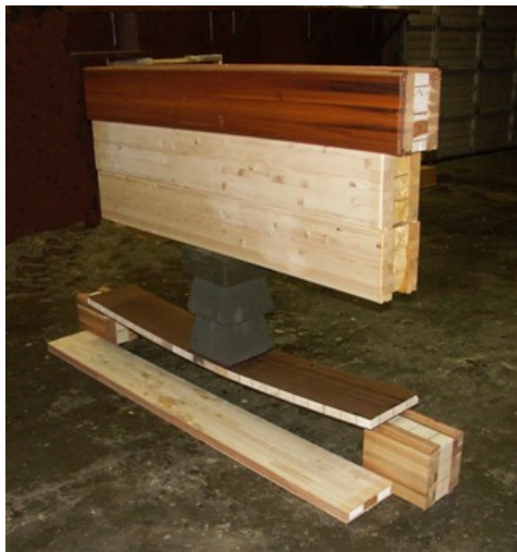
1 3/4" thick Sing Honeycomb with same facial material as paper honeycomb
